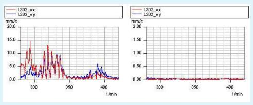
Cavern head vibrations during initial state (left) and after modification (right).
