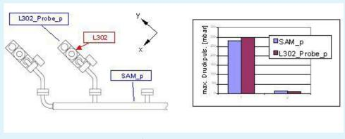
Positions of pressure (blue) and vibration measuring points (red) at the cavern head as well as maximum pressure pulsations, initial state (1) and modification (2).
