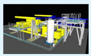
Modification by installing a vertical two-chamber damper.
